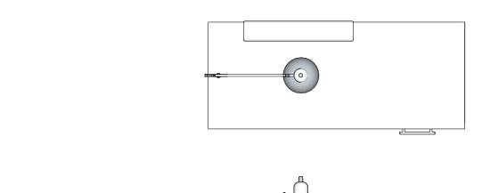
There is no power strip or outlet included with this unit. Electrician to provide, install, and wire a 15 amp outlet installed in the wall or floor within reach of the lamp's 59" long cord.
