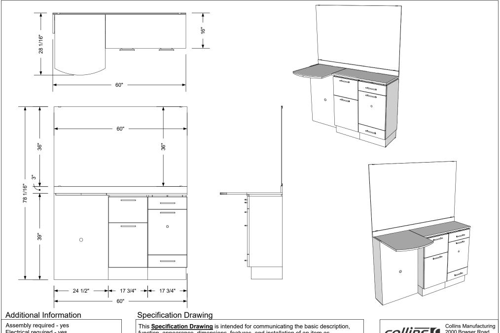
Electrical required - yes Plumbing required - yes Wall blocking required - no COM yardage/laminate usage - 57 sf 5 1/2"h laminated toe + 1/4"h glides Other (specify) - n/a Other (specify) - n/a
