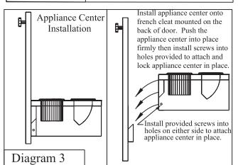
BackSplash/ by using provided mending plates or by using contractor's adhesive. If using mending plates, attach mending plates to Mending Plate backsplash then to the cabinet using the screws provided. Installation See diagram below. Diagram 6 French cleat detail French cleat should be attached to the
