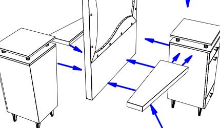
STEP 2. Mount each purse ledge to mirror frame with (3) 1 1/2" hex head bolts through ledge into t-nuts in the mirror frame.
