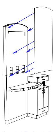
Step 4: Install mirrors by following the directions on the mirror clip boxes. Mirrors should be mounted in 2" from sides and 2" above ledge.
