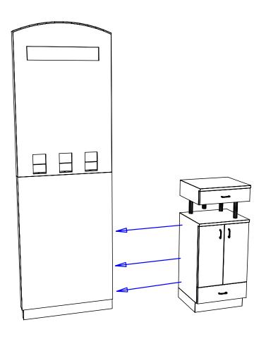
Step 2: Bolt though the pre-drilled holes on the interior of the Base cabinet into the lower wall. Use the provided 1 1/2" hex head bolts and washers. There are three bolts for each base cabinet.
