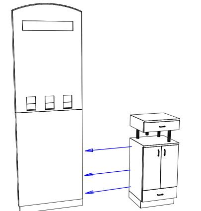
Step 2: Bolt though the pre-drilled holes on the interior of the Base cabinet into the lower wall. Use the provided 1 1/2" hex head bolts and washers. There are three bolts for each base cabinet.
