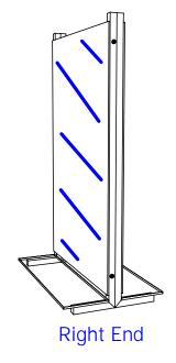
These drawings show the orientation of the holes drilled in the metal frame for attachment to the individual stations. Also note the placement of the preinstalled brackets on the wood panel. To attach the L/R of the mirror frame to center panel drive screws into the predrilled holes.
