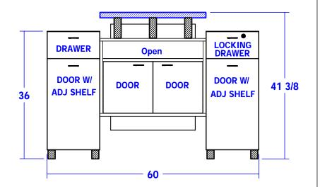
This cabinet is shipped fully assembled. No further assembly or installation is required.
