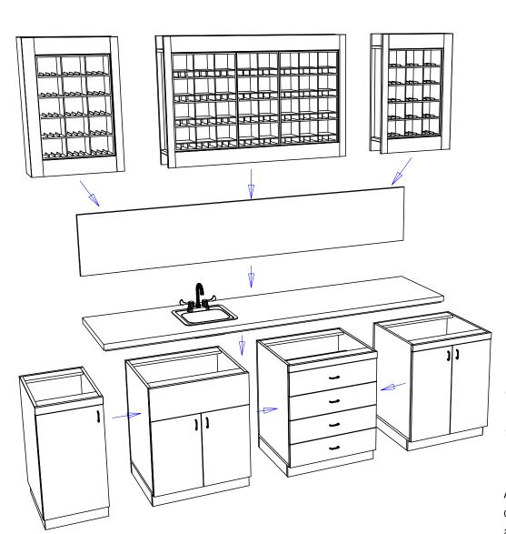
Attach adjacent cabinets by fastening through the pre-drilled holes with the provided connector bolts and matching connector nut.
