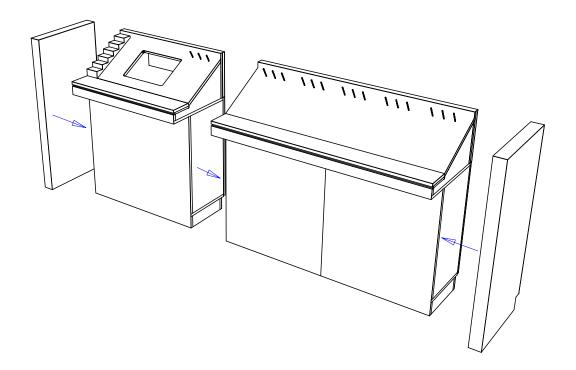
Attach adjacent cabinets, end panels, and support legs by fastening through the pre-drilled holes with the provided connector bolts. These bolts will thread into a factory installed threaded fastener, t-nut or provided matching connector nut depending upon the application and visibility of the fasteners. Some applications may require drilling holes on-site and the use of 1 ¼" wood screws and decorative washers.
