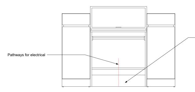
Provide 20 amp electrical stub within the footprint of the front panel. The power may then be directed through the lower shelf and connected to an outlet. The outlet is provided, installed, and wired by the electrician according to project-specific requirements.
