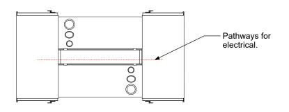
The island includes 20 amp fourplex outlets mounted below the countertop on both inboard ends of the cabinets. The tools plug into these outlets.
