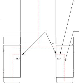
The electrician is responsible for connecting power to the fourplex outlets up from the floor or down from the ceiling along the indicated path. Provide a 20 amp, switched outlet for each student station (two per double island).
