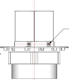
The guad island includes 20 amp fourplex outlets mounted below the mirror on all six faces of the station. The tools plug into these outlets.
