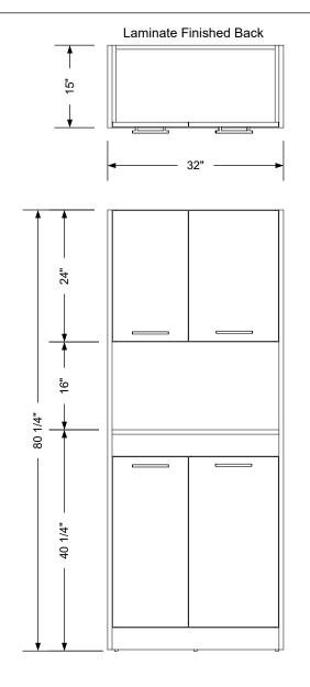
For free-standing installation, Collins recommends anchoring the unit to the floor with floor blocking.
