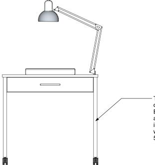
There is no power strip or outlet included with this unit. Electrician to provide, install, and wire a 15 amp outlet installed in the wall or floor within reach of the lamp's 59" long cord.
