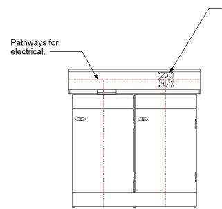
The electrician is responsible for connecting power to the fourplex outlets at the indicated location. Provide a 20 amp circuit for each outlet. Outlets are provided by Collins.
