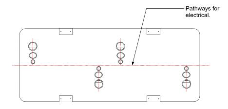
Electrical may stub out at the wall and run through adjacent stations or it may stub from the floor and branch off to power the other stations. Grommet are provided in the support legs.
