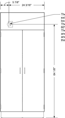
The prewired power cord exits the wig dryer in this location in the back.
