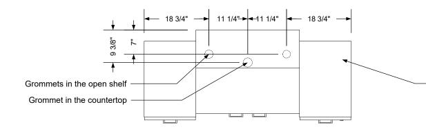
Provide 20 amp electrical power into the cabinets either through the bottom or end of one of the two cabinets. The power may then be directed through the desk and connected to outlets. The outlets are provided, installed, and wired by the electrician according to project-specific requirements.
