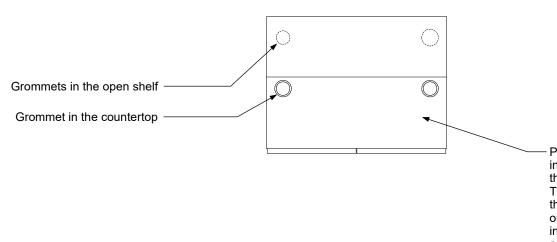
Provide 20 amp electrical power into the cabinets either through the bottom or side of the cabinet.
