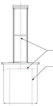
The electrician is responsible for connecting power to the fourplex outlets either from the floor or down from the ceiling, or from station to station along the indicated path. Provide a 20 amp, switched outlet for each student (two per island station).
