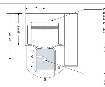
Water supply connections and drain connections can easily be made as long as the stub outs fall within the footprint or back profile of the seat support box. The plumber is responsible for providing the appropriate components and supply lines.
