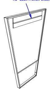
French cleat should be attached to the wall by screwing through the cleat into wall stud or blocking using the fasteners provided. The cleat should be level and at the indicated height.
