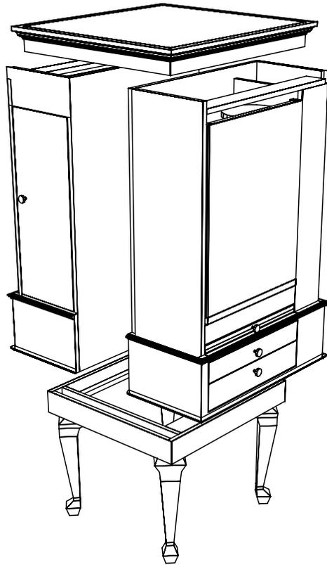
**Set base unit with legs in the desired location then set the upper cabinets on top of the base. Then anchor the cabinets by screwing up through the base.**
