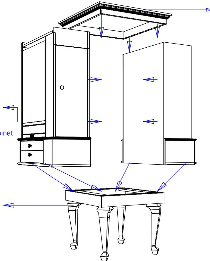
STEP 3. Place crown cap on top of cabinets and fasten using (4) 1 1/2" wood screws in each corner. Screw down through cap into cabinets.
