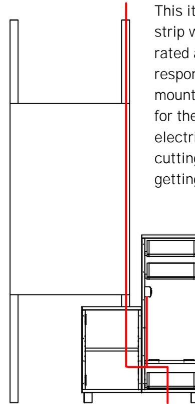
This item includes a six outlet power strip with a 4' cord. The outlet strip is rated at 15 amps. The electrician is responsible for providing and mounting an outlet inside the cabinet for the power strip to plug into. The electrician is also responsible for cutting an appropriate entry point for getting power into the cabinet.
