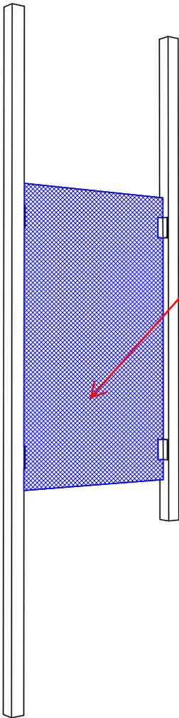
Match panel "A" with steel posts also marked with an "A" -- B to B, etc
