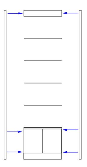
This item is attached to the wall with wood screws. 3" wood screws and decorative washers are provided for wood framed walls. Fasteners for other wall types are to be obtained locally. Screw through the back panel in locations which will be inconspicuous after installation. Suggested locations include: under shelves, behind drawers, and locations hidden by products or supplies.
