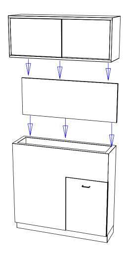
This item is attached is attached to the wall with wood screws. 3" wood screws and decorative washers are provided for wood framed walls. Fasteners for other wall types are to be obtained locally. Screw through the back panel in locations which will be inconspicuous after installation. Suggested locations include: under shelves, behind drawers, and locations hidden by products or supplies.
