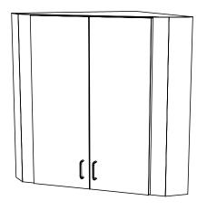
This item is attached to the wall with wood screws. 3" wood screws and decorative washers are provided for wood framed walls. Fasteners for other wall types are to be obtained locally. Screw through the back panel in locations which will be inconspicuous after installation. Suggested locations include: under shelves, behind drawers, and locations hidden by products or supplies.
