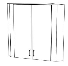
This item is attached to the wall with wood screws. 3" wood screws and decorative washers are provided for wood framed walls. Fasteners for other wall types are to be obtained locally. Screw through the back panel in locations which will be inconspicuous after installation. Suggested locations include: under shelves, behind drawers, and locations hidden by products or supplies.
