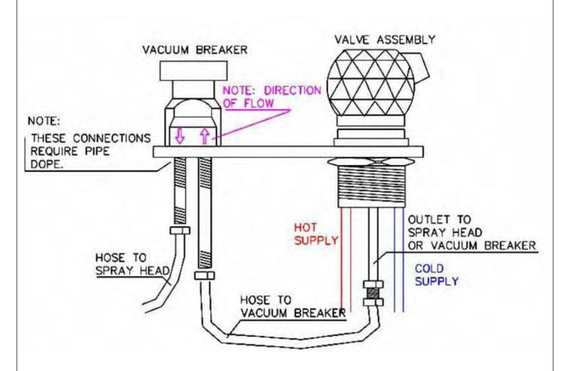
Note arrows on the vacuum breaker that indicate directional flow of water.
