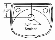
Fasten mounting plate to wall. Place bowl on top of plate flange with back side of bowl against leveling bolt. Use two 5/16" - 18 x 1/2" rd. hd. screws with 3/8" x 1" washers to fasten plate flange to underside of shampoo bowl. (Do not overtighten.)
