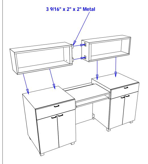
Use the provided 1 1/4" Decorative bolts to bolt the upper cabinets to each other. Do not tighten the bolts. Use the Provided 1 1/4" hex bolts and washers to bolt through the interior top of the base cabinets into the bottom of the upper cabinets. Once all bolts have been started go back and firmly tighten the bolts.
