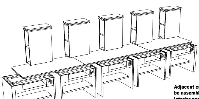
Duplex and quad outlets are provided with 15 amp grounded receptacles. Electrician should provide power supply and connect to receptacles per local and national electric codes.
