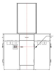
The quad island includes 20 amp fourplex outlets mounted below the tool panel on the rights ends of all four cabinets. The tools plug into these outlets.
