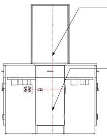
The electrician is responsible for connecting power to the fourplex outlets up from the floor or down from the ceiling along the indicated path. Provide a 20 amp, switched outlet for each student station (four per quad island island).
