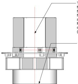
The electrician is responsible for connecting power to the fourplex outlets up from the floor or down from the ceiling along the indicated path. Provide a 20 amp, switched outlet for each student station (six per hex station).
