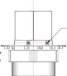
The quad island includes 20 amp fourplex outlets mounted below the mirror on all six faces of the station. The tools plug into these outlets.
