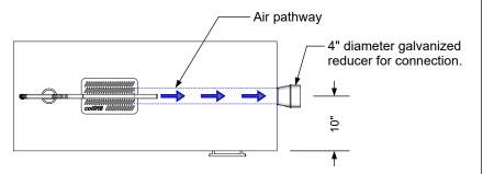
All connnections from the nail table to the ventilation system to be provided and installed by others. All air movement calculations and air handling systems to be provided by HVAC contractor.
